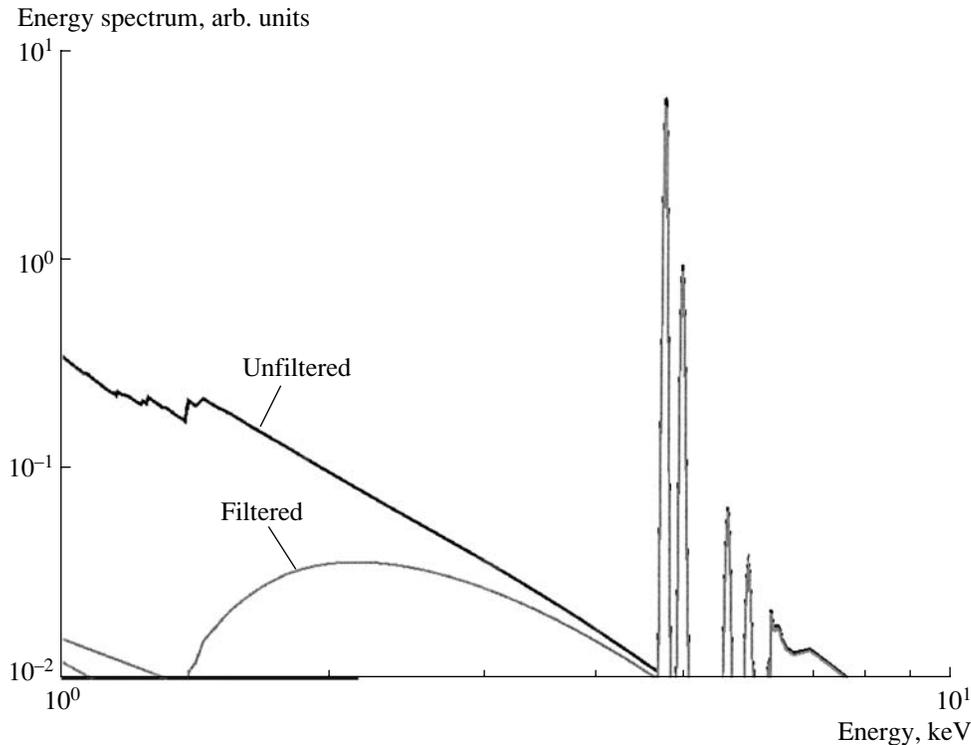
**Fig. 3.** X-ray spectrum of a Ti z-pinch on the Z machine at Sandia National Laboratories. The raw PRS spectrum (black line) is compared to the 0.5 mm Li-metal shielded measurement (grey line).
