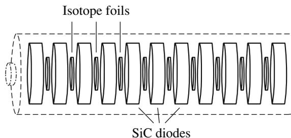
**Fig. 1.** Schematic of a conceptual nuclear battery in AA format.
