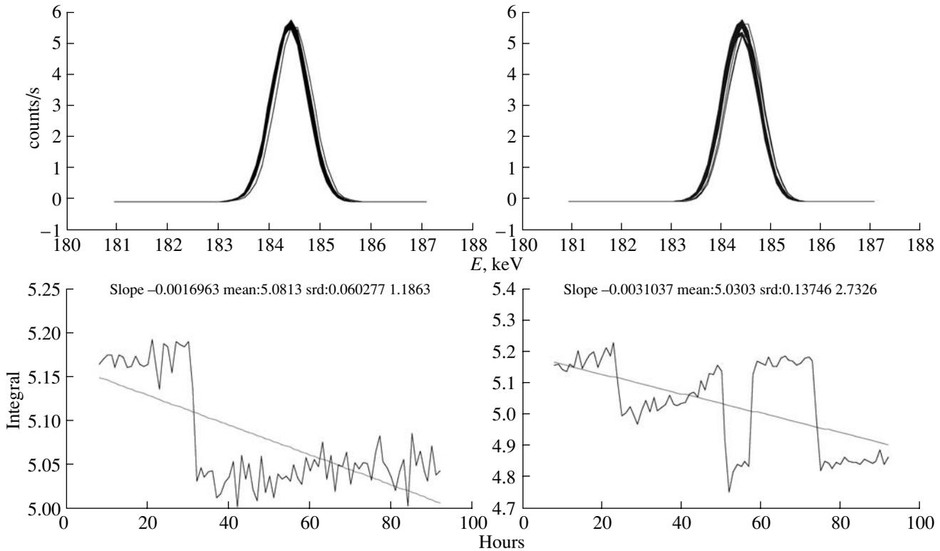
**Fig. 5.** Hourly count in the 184.41 keV line over ~90 h before irradiation (left). The same  $\gamma$  line after a 39 h bremsstrahlung irradiation with  $3 \times 10^{12}$  photons/s/cm<sup>2</sup> (right).
