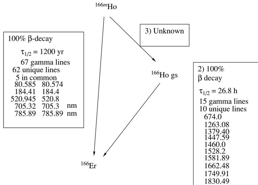
Fig. 3. Decay path of  $^{166m}\text{Ho}$ .
