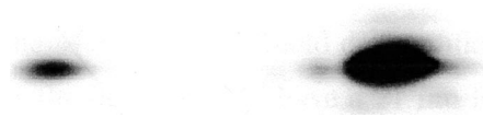
FIG. 4. X-ray image of 10 \mu\text{m} beam (left-hand side) with 10 \times longer exposure time (right-hand side).
