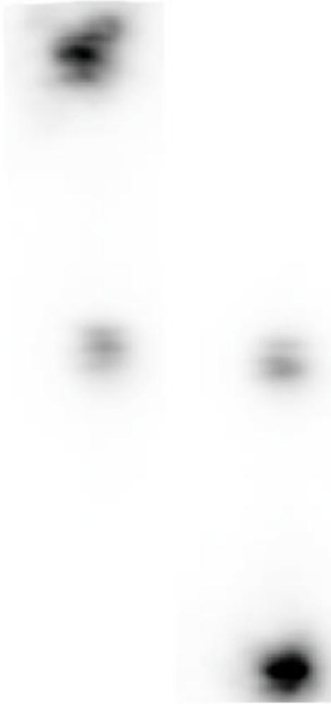
**Figure 7.** A nominally  $20\ \mu\text{m}$  square x-ray beam focused by the lens  $200\ \mu\text{m}$  above (left image) and below the optical axis (right image).
