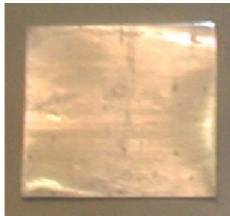
FIG. 1. (Color online) Square foil of 0.28 mm thick Li–LiH, 60 mm on both sides.
