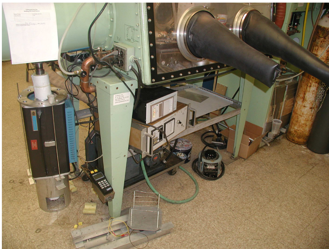
FIG. 3: Parylene coater connected to the glove box in NRL's building 256.
