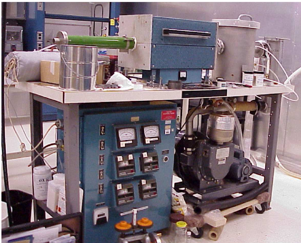
FIG. 2: Parylene coater setup in the dry room of ARL's building 207.
