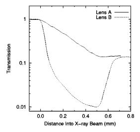
FIG. 3. Transmission of a 30  $\mu$ m beam through a jaw as it is inserted into the beam, while held parallel to the beam. Lens A is handled properly, in dry nitrogen and then under a constant vacuum. Lens B's transmission decreases 1 order of magnitude faster, due to corrosion from water vapor that was introduced by a leaky seal.
