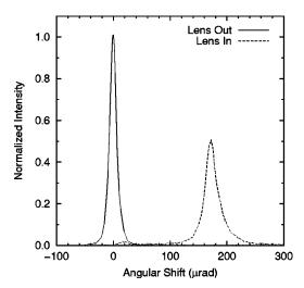
FIG. 4. A slice through a CCD image before and after the lens is inserted into the  $30 \mu m$  beam. The large peak for when the lens is in the beam is due to the first harmonic 10 keV photons, while the tiny peak is due to the third harmonic 30 keV photons.
