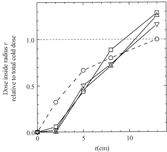
Fig. 13. Dose distributions measured with collimated PD detectors relative to the total dose for a shot with an unheated anode (circles). The cathode tip axes are located at  $r = 8$  cm, and the anode rods are at  $r = 13$  cm. Data for three shots with hot anodes are indicated by squares and triangles.
