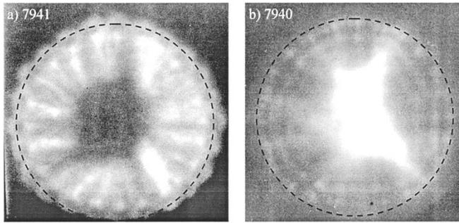
Fig. 12. Time-integrated X-ray pinhole photographs of (a) hot and (b) unheated tantalum anodes using the stretching mechanism. The axes of the cathode tips lie on the dashed circles [see Fig. 11(c)].
