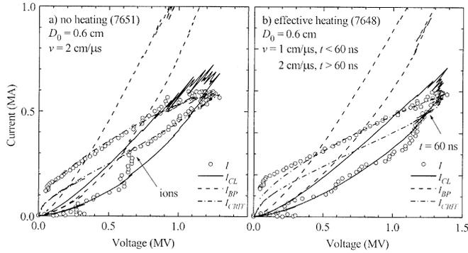
Fig. 7. Current–voltage characteristics (circles, 1 ns/point) compared with diode models (lines) for (a) unheated and (b) heated anodes. Model parameters are  $r = 6$  cm,  $\Delta r = 3$  mm, initial A–K gap  $D_0$ , and gap-closure velocity  $v$ .
