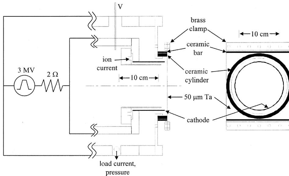
Fig. 3. Tantalum heating setup on Gamble II. The generator is represented by its characteristic impedance ( $2 \Omega$ ) and open-circuit voltage waveform (maximum 3 MV). The vacuum diode consists of a hollow cylindrical cathode and a rectangular tantalum foil stretched over ceramic structures for thermal and electrical isolation during heating. The locations of voltage, current, ion current, and pressure measurements are indicated.
