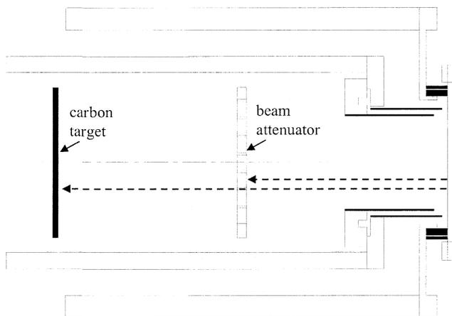
Fig. 9. Setup used to detect high-energy protons by carbon activation. The attenuator is located 22 cm from the tantalum anode and the carbon target is located 44 cm from the tantalum anode. Dashed lines indicate typical proton trajectories.
