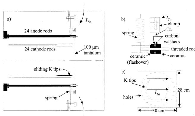
Fig. 11. Sketch of the tantalum-stretching mechanism. (a) Top view cross section, (b) close up of clamping assembly, and (c) front view of tantalum foil.
