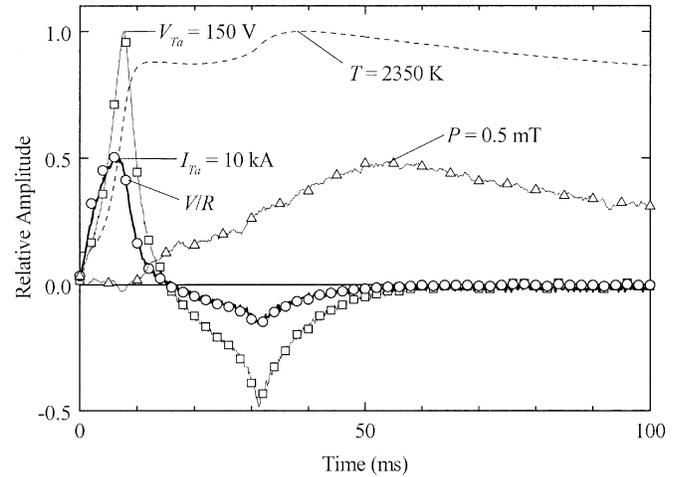
Fig. 2. Heating analysis based on measured voltage ( $V_{Ta}$ , squares) and current ( $I_{Ta}$ , thick line) for a  $16.5 \text{ cm} \times 18 \text{ cm} \times 50 \mu\text{m}$  tantalum foil driven by a capacitor-bank discharge. Calculated temperature ( $T$ , broken line) determines resistance  $R$  used to compare  $V/R$  (circles) with measured current. Pressure ( $P$ , triangles) increases after the foil is heated.
