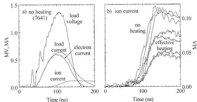
Fig. 6. Electrical data for (a) a shot with no heating and (b) ion current signals for shots with heating (squares) and without heating (lines). Electron current is the difference between the measured load current and ion current.
