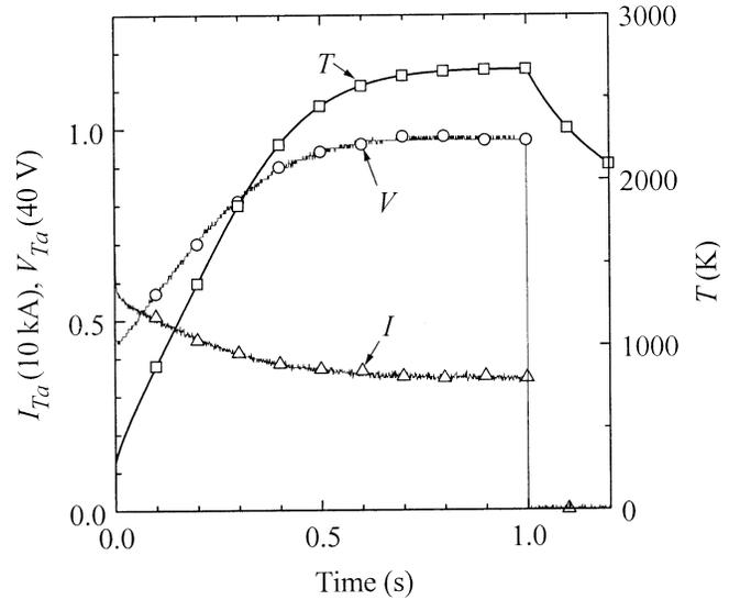
Fig. 8. Measured voltage (circles) and current (triangles) for heating a  $28$  cm  $\times$   $30$  cm  $\times$   $100$   $\mu$ m tantalum foil with a battery bank. The calculated temperature (squares) exceeds  $2600$  K.
