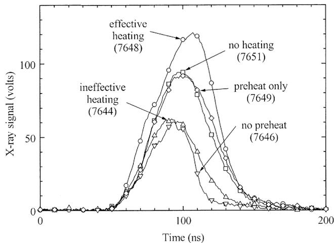
Fig. 4. X-ray (PD) signals using different heating procedures: no heating (squares), effective heating (circles), ineffective heating (up triangles), no preheat (down triangles), and preheat only (diamonds).
