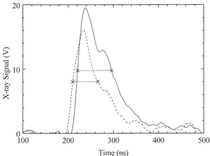
Fig. 14. Comparison of X-ray signals from DM2 for shots with hot (shot 839, solid line) and unheated (shot 838, dashed line) anodes. Horizontal lines with crosses indicate the FWHM. Time zero corresponds to the start of the generator current, upstream of the POS.
